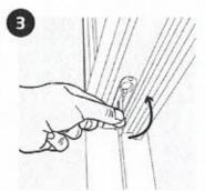
To close the door, simply move the door back into the frame and push the shoot bolts back to the original position.
