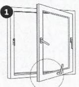
The wind-brake restrictor is found at the bottom of the frame when window is open in cleaning position.
