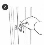
Release the central mullion lock by holding down the control button and turning the handle inwards
