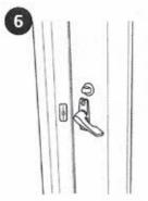
To close the door, ensure the handle is pointing downwards and the central mullion lock is disengaged
