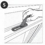
Disengage the stay on the top rail of the sash, by sliding the sash to the hinge side of the window.
